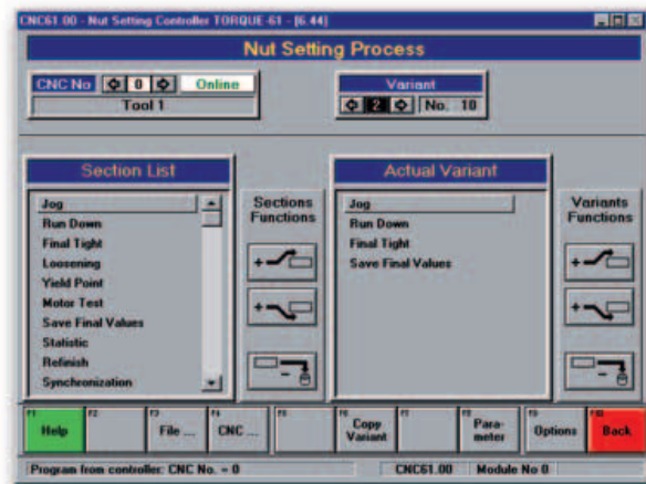
Any nut setting processes can be created by selecting sections from a list.
